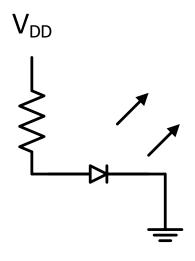
If VDD is 3.3V and the resistor is 1.0K $\Omega$ , then according to Ohm's Law, the maximum current through the LED is I = V/R = 3.3/1000 = 0.0033 Amps = 3.3 mA
